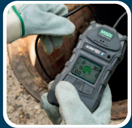
Gas Free Testing Safe environments for hot work
